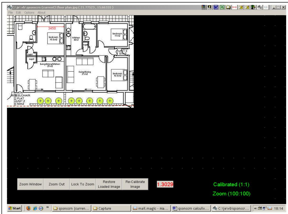
To illustrate Calculix mode, load the image “floor plan.jpg” then zoom in and calibrate it using the 3.45m length shown in one of the bedrooms.
